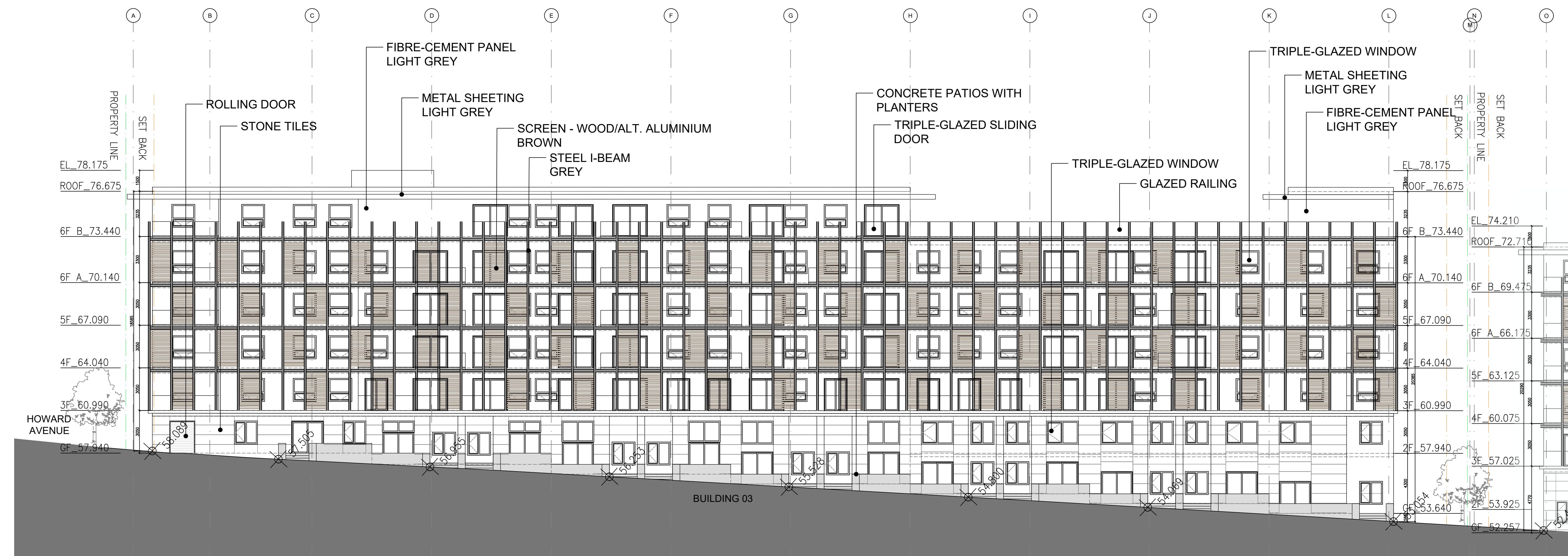
2 SOUTH ELEVATION- BLDG 3 A3.03 1:150
